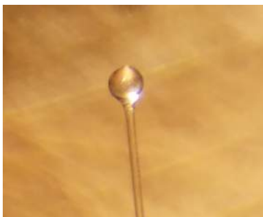
FIGURE 3.1. Image of a fused silica microsphere, approximately 75 \mu\text{m} in diameter. This sphere was fabricated by slowly feeding and rotating a thin fiber stem (produced by etching a Corning SMF-28e+ fiber in Hydrofluoric acid to \approx 20\mu\text{m} diameter) into the electrical arc of a fusion splicer.
